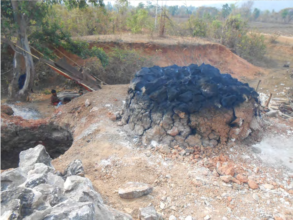
Fig. 18: Lime stove in operation: The vertical hole for the fire and the horizontal hole filled with lime stones
